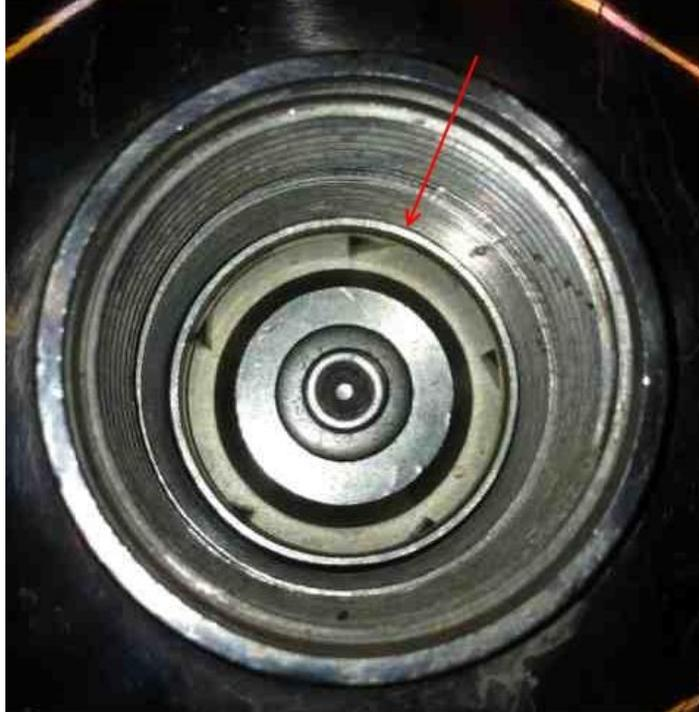
3.15 Rotate the impeller by hand to be sure it is not rubbing. This can be done by sticking your finger in the discharge nozzle and rotating the impeller or with a screwdriver placed in the back of the motor.
