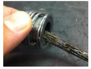
3.08 Place the rotating half of the seal gently over the shaft. Do not scratch the seal face. Press down with your thumbs and slide the seal over the shaft. Do not press the seal past the shoulder of the motor shaft.
