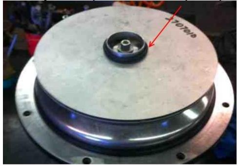
For pump using the stainless steel baseplate, skip to step 3.13. For 3 phase motors: Place the case on the top of the assembly. The 8 bolt holes on the flange should line up with the 8 bolt holes in the sealplate and adapter plate. Thread the 8 case screws down by hand to ensure the threads in the adapter plate are in good condition. This also helps reduce occurrences of galling. Tighten the 8 case bolts to approximately 8 ft-lbs.
