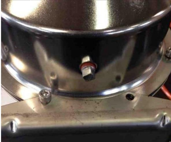
Place the case onto the sealplate, over the o-ring.
