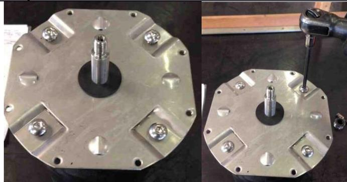
Install the 4 motor mounting bolts by hand. This prevents the threads from galling or breaking with installation using an air ratchet.
