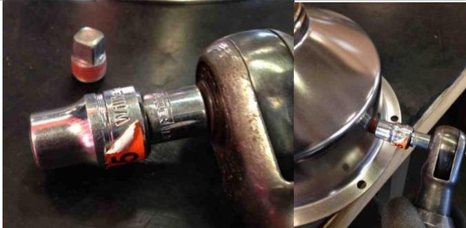
**Install the Drain Plug into the Case**
