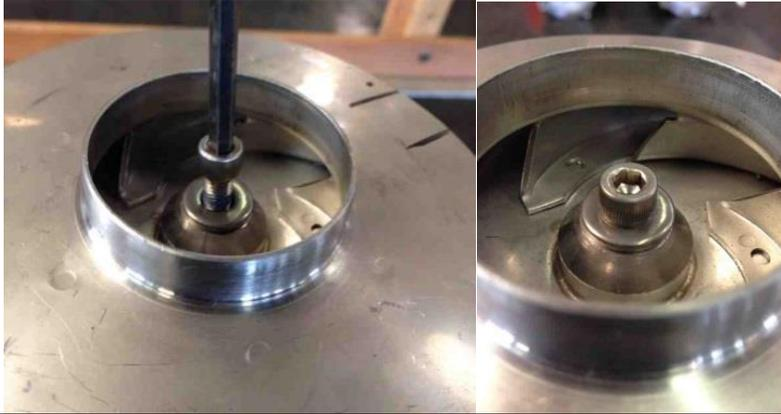
**Installing the Locking Screw and Washer**
