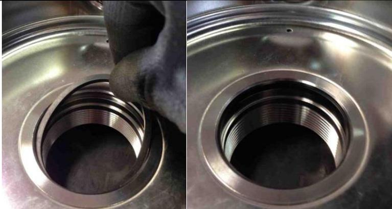
**Installing the Suction O-Ring**
