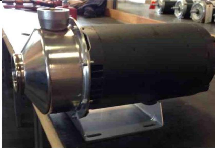
A completed pump assembly with a stainless steel baseplate can be seen in the picture on the left
