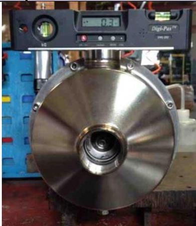
The top of the suction nozzle must be level with the ground. If the suction nozzle threads are crooked, it may not fit into the customers' system if hard piped.
