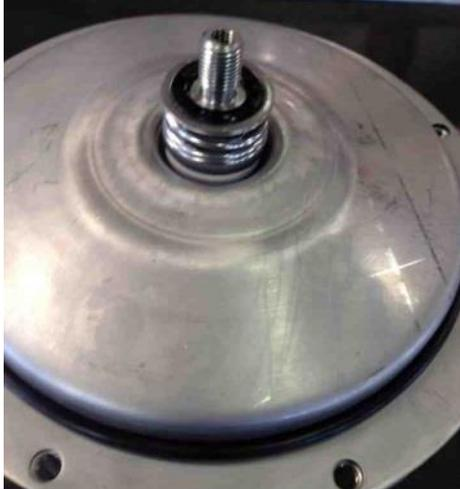
Install the o-ring onto the sealplate as shown in the picture. The o-ring should not be twisted or rolled.
