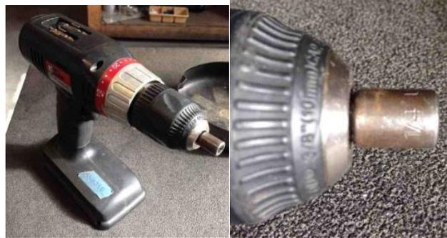
Electric Drill (for removing wire cover screws)
