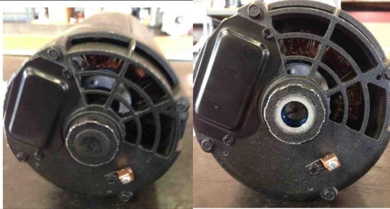
The motor manufacturer supplies a plug in the back of the motor. It can be seen in this picture as a black plug at the center of the motor.
